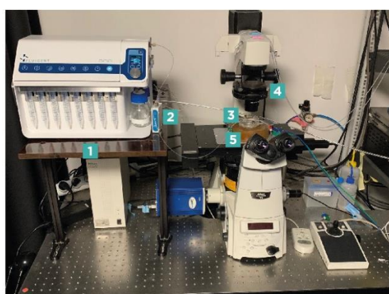
Figure 1: System setup. Aria and a valve are connected to the EPHESIA microfluidic chip. The 10 solutions to be injected are present inside the reservoirs.
