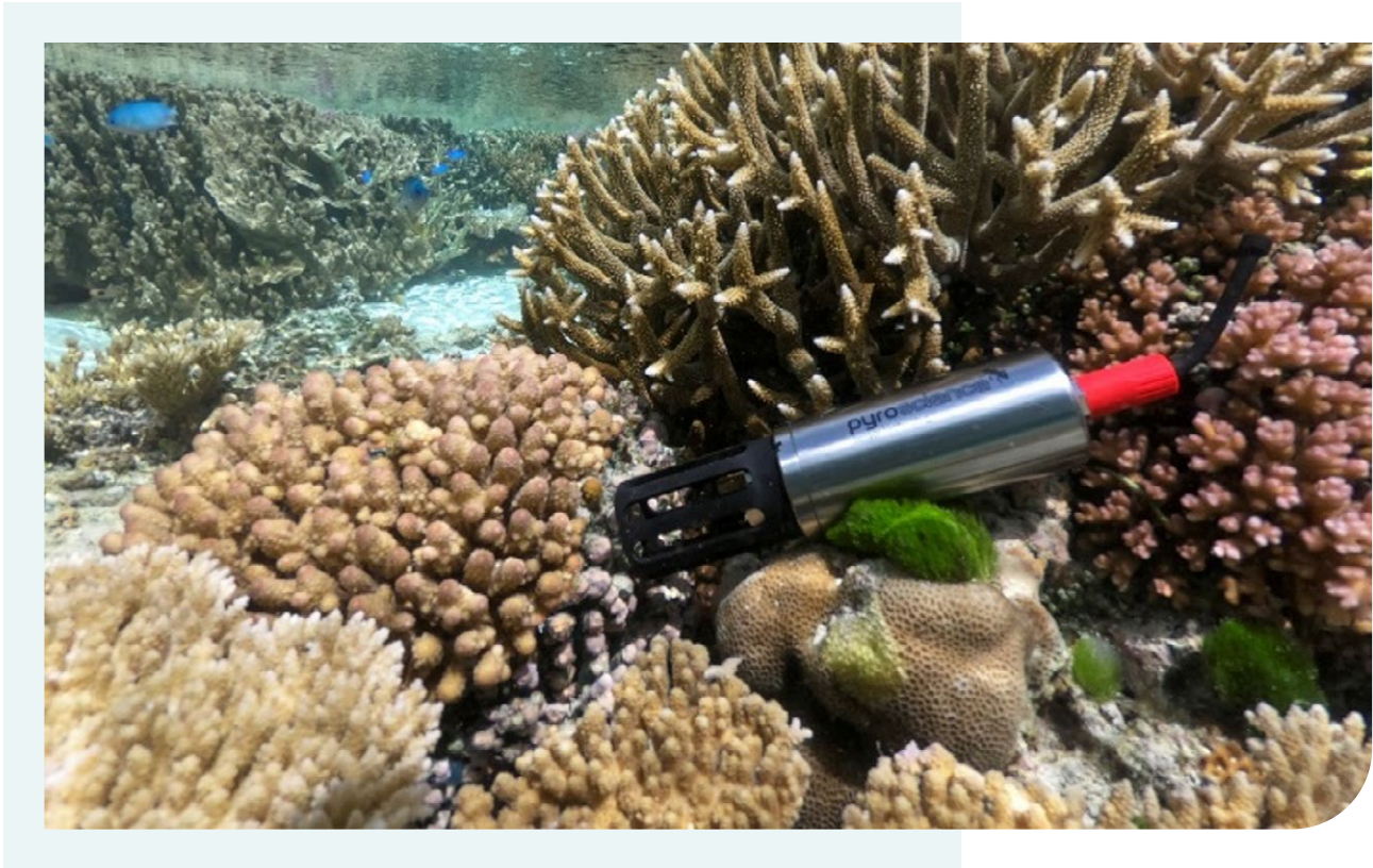
AquapHOx instrument for long-time monitoring of Oxygen and pH in shallow water and down to 4000m water depth.
