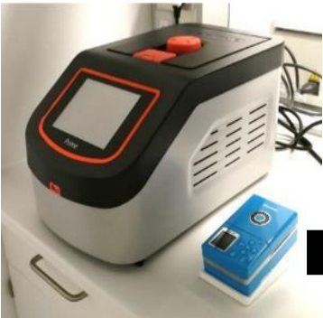
Conventional thermocycler vs cPCR cycler (1500bp: 2hours vs. 30min)
