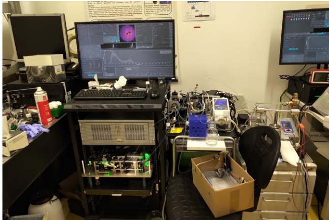
BRAVE B1 sensor-station (open detector unit), monitoring SiC lab-scale CNANO particles with H.A.N.S. software suite (top); right: continuous dilution system for on-line measurement including continuous ultrasonication..
